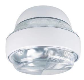
The first of several surface mounted fixtures by ELA, the *Carlsbad* offers durability, aesthetics, and performance. Built from quality grade extruded aluminum, the low profile design offers the perfect solution for many overhead applications. The dropped prismatic refractive lens produces wide, uniform optics for a greater fixture spread.
